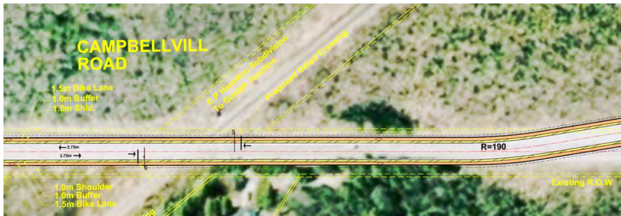
Exhibit 20-7: Railway Crossing Alteration on Campbellville Road
