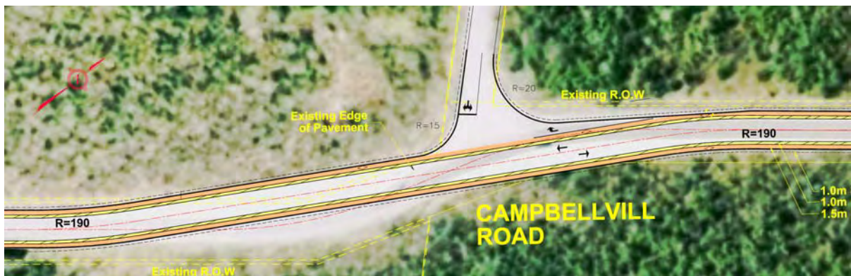
Exhibit 20-6: Horizontal Alignment Alteration on Campbellville Road
